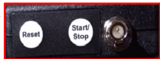
Start/Stop and Reset buttons found on top of Dolphin Wireless Start Unit.
